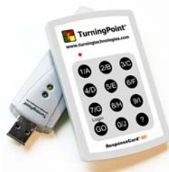
Figure 1. Personal Response Unit (Clicker) and USB Receiver
