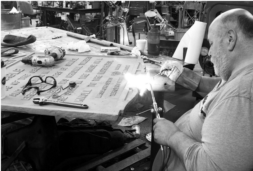
Leo Levesque uses a brazing rod to pour molten metal into the cracks. The surface was then ground down again, and sent back to the sand-blaster, so that the sign's surface would have an even texture.
