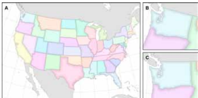
↑ Figure 1: When using the Lambert conformal conic map projection for the US (A), which is centered on 96 degrees west longitude, a map of Washington (B) will appear tilted. Changing the central meridian of the map projection to -120 (the approximate east-west center of the state) will fix the problem (C).
