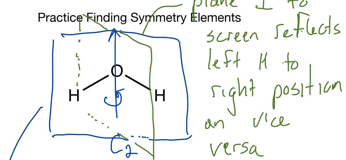
atoms all contained in the plane of the screen. If the screen is a mirror, the back halves would be reflected to the front halves
