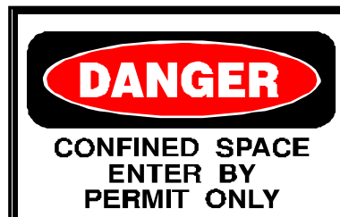
Figure 1: Sign to Satisfy Requirements of §1910.146(c)(2)
